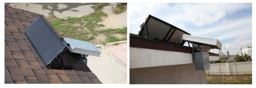
AirBase Multi-Sensor Air Quality Monitoring Station Version I CFASE Designed Solar Panel Renewable Energy Source & 8 Hour - 12 VDC Backup Battery Supply
