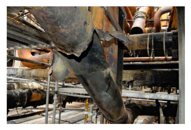
Figure 7. Photo of rupture on 4-sidecut 52-inch component.
