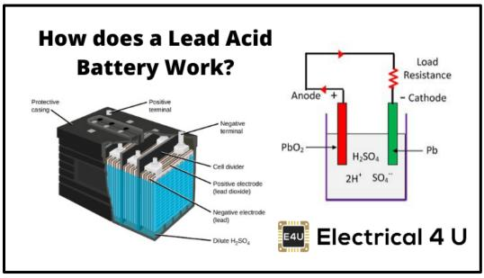
Figure 2-5 Lead-Acid Battery Components
