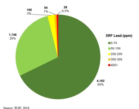
Figure 3.4-2 Results from Soil Samples at Residential Properties
