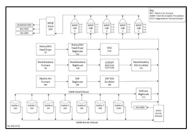
The facility's air pollution control systems operate continuously and are inspected daily, as required by applicable South Coast AQMD permits and regulations. Routine checks look for
