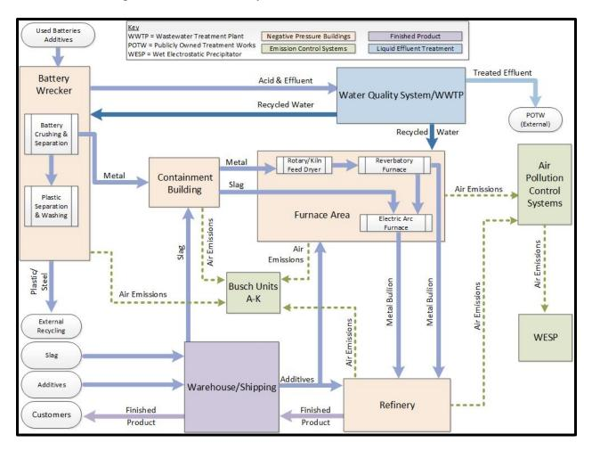
Figure 2-6 Overview of Quemetco's Lead Recycling Process, Products, and Discharges
