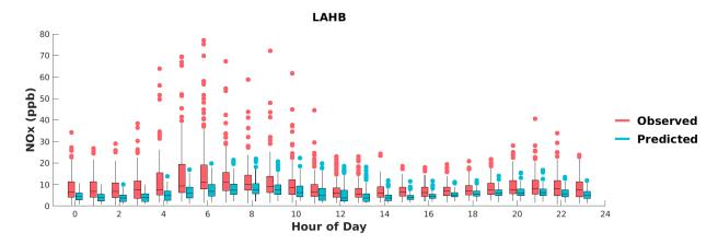
FIGURE I-10: BOX PLOTS OF OBSERVED VS. PREDICTED HOURLY NOX DURING MAY 1<sup>ST</sup> TO SEPTEMBER 30<sup>TH</sup>, 2018, AT LA HABRA. HORIZANTAL LINES INDICATE 25<sup>TH</sup>, 50<sup>TH</sup> (MEDIAN), AND 75<sup>TH</sup> PERCENTILES.
