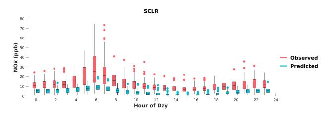
FIGURE I-19: BOX PLOTS OF OBSERVED VS. PREDICTED HOURLY NOX DURING MAY 1<sup>ST</sup> TO SEPTEMBER 30<sup>TH</sup>, 2018, AT SANTA CLARITA. HORIZANTAL LINES INDICATE 25<sup>TH</sup>, 50<sup>TH</sup> (MEDIAN), AND 75<sup>TH</sup> PERCENTILES.
