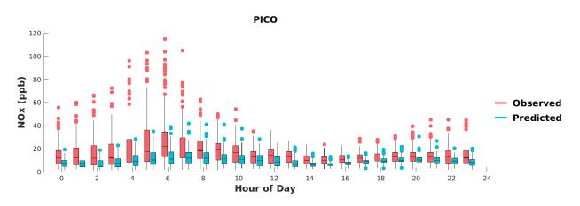
FIGURE I-14: BOX PLOTS OF OBSERVED VS. PREDICTED HOURLY NOX DURING MAY 1<sup>ST</sup> TO SEPTEMBER 30<sup>TH</sup>, 2018, AT PICO RIVERO. HORIZANTAL LINES INDICATE 25<sup>TH</sup>, 50<sup>TH</sup> (MEDIAN), AND 75<sup>TH</sup> PERCENTILES.
