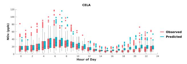
FIGURE I-4: BOX PLOTS OF OBSERVED VS. PREDICTED HOURLY NOX DURING MAY 1<sup>ST</sup> TO SEPTEMBER 30<sup>TH</sup>, 2018, AT CENTRAL LOS ANGELES. HORIZANTAL LINES INDICATE 25<sup>TH</sup>, 50<sup>TH</sup> (MEDIAN), AND 75<sup>TH</sup> PERCENTILES.
