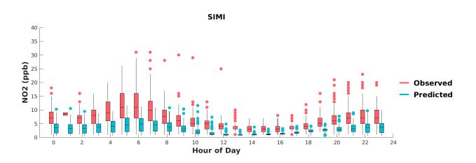
FIGURE H-20: BOX PLOTS OF OBSERVED VS. PREDICTED HOURLY NO2 DURING MAY 1<sup>ST</sup> TO SEPTEMBER 30<sup>TH</sup>, 2018, AT SIMI VALLEY. HORIZANTAL LINES INDICATE 25<sup>TH</sup>, 50<sup>TH</sup> (MEDIAN), AND 75<sup>TH</sup> PERCENTILES.
