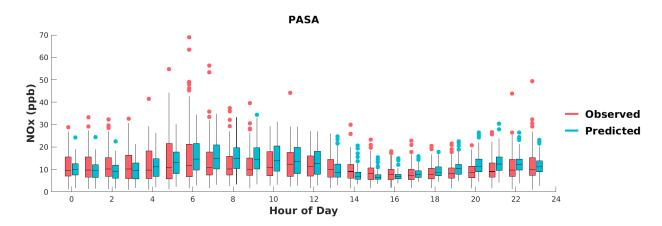
FIGURE I-13: BOX PLOTS OF OBSERVED VS. PREDICTED HOURLY NOX DURING MAY 1<sup>ST</sup> TO SEPTEMBER 30<sup>TH</sup>, 2018, AT PASADENA. HORIZANTAL LINES INDICATE 25<sup>TH</sup>, 50<sup>TH</sup> (MEDIAN), AND 75<sup>TH</sup> PERCENTILES.
