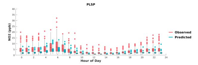
FIGURE H-16: BOX PLOTS OF OBSERVED VS. PREDICTED HOURLY NO2 DURING MAY 1<sup>ST</sup> TO SEPTEMBER 30<sup>TH</sup>, 2018, AT PALM SPRINGS. HORIZANTAL LINES INDICATE 25<sup>TH</sup>, 50<sup>TH</sup> (MEDIAN), AND 75<sup>TH</sup> PERCENTILES.
