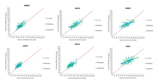
FIGURE K-1: SCATTER PLOT OF OBSERVED VS. PREDICTED MDA8 OZONE DURING MAY 1<sup>ST</sup> TO SEPTEMBER 30<sup>TH</sup>, 2018, AT ANEHIM (ANAH), AZUSA (AZUS), BANNING (BANP), COMPTON (CMPT), CENTRAL LOS ANGELES (CELA), AND CRESTLINE (CRES). GREEN AND BLUE LINES INDICATE GENERAL LINEAR MODEL FIT WITH 95% CONFIDENCE INTERVAL (SHADED AREA). THE RED LINE INDICATES 1:1 LINE.
