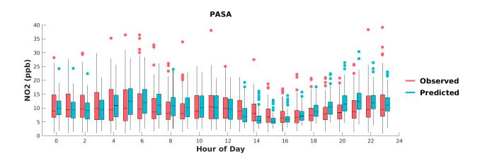
FIGURE H-13: BOX PLOTS OF OBSERVED VS. PREDICTED HOURLY NO2 DURING MAY 1<sup>ST</sup> TO SEPTEMBER 30<sup>TH</sup>, 2018, AT PASADENA. HORIZANTAL LINES INDICATE 25<sup>TH</sup>, 50<sup>TH</sup> (MEDIAN), AND 75<sup>TH</sup> PERCENTILES.
