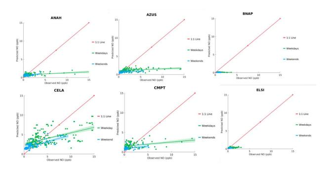
FIGURE L-1: SCATTER PLOT OF OBSERVED VS. PREDICTED DAILY AVERAGE NO DURING MAY 1<sup>ST</sup> TO SEPTEMBER 30<sup>TH</sup>, 2018, AT ANEHIM (ANAH), AZUSA (AZUS), BANNING (BANP), COMPTON (CMPT), CENTRAL LOS ANGELES (CELA), AND LAKE ELSINORE (ELSI). GREEN AND BLUE LINES INDICATE GENERAL LINEAR MODEL FIT WITH 95% CONFIDENCE INTERVAL (SHADED AREA). THE RED LINE INDICATES 1:1 LINE.
