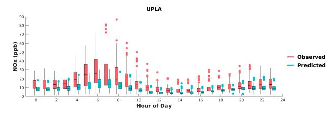
FIGURE I-22: BOX PLOTS OF OBSERVED VS. PREDICTED HOURLY NOX DURING MAY 1<sup>ST</sup> TO SEPTEMBER 30<sup>TH</sup>, 2018, AT UPLAND. HORIZANTAL LINES INDICATE 25<sup>TH</sup>, 50<sup>TH</sup> (MEDIAN), AND 75<sup>TH</sup> PERCENTILES.
