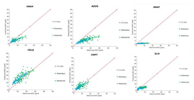
FIGURE M-1: SCATTER PLOT OF OBSERVED VS. PREDICTED DAILY AVERAGE NO2 DURING MAY 1<sup>ST</sup> TO SEPTEMBER 30<sup>TH</sup>, 2018, AT ANAHEIM (ANAH), AZUSA(AZUS), BANNING (BNAP), CENTRAL LOS ANGLES (CELA), COMPTON (CMPT), AND LAKE ELSIONOR (ELSI). GREEN AND BLUE LINES INDICATE GENERAL LINEAR MODEL FIT WITH 95% CONFIDENCE INTERVAL (SHADED AREA). THE RED LINE INDICATES 1:1 LINE.
