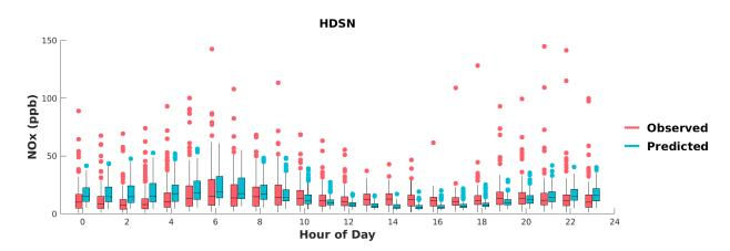
FIGURE I-9: BOX PLOTS OF OBSERVED VS. PREDICTED HOURLY NOX DURING MAY 1<sup>ST</sup> TO SEPTEMBER 30<sup>TH</sup>, 2018, AT HUDSON. HORIZANTAL LINES INDICATE 25<sup>TH</sup>, 50<sup>TH</sup> (MEDIAN), AND 75<sup>TH</sup> PERCENTILES.
