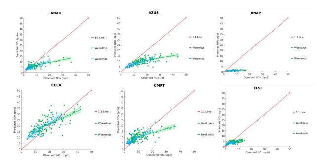
FIGURE N-1: SCATTER PLOT OF OBSERVED VS. PREDICTED DAILY AVERAGE NOX DURING MAY 1<sup>ST</sup> TO SEPTEMBER 30<sup>TH</sup>, 2018, AT ANEHIM (ANAH), AZUSA (AZUS), BANNING (BANP), COMPTON (CMPT), CENTRAL LOS ANGELES (CELA), AND LAKE ELSINORE (ELSI). GREEN AND BLUE LINES INDICATE GENERAL LINEAR MODEL FIT WITH 95% CONFIDENCE INTERVAL (SHADED AREA). THE RED LINE INDICATES 1:1 LINE.
