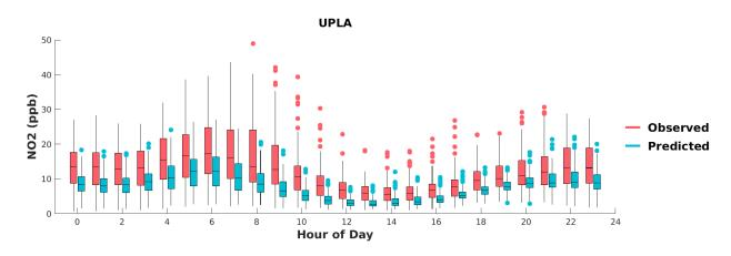
FIGURE H-22: BOX PLOTS OF OBSERVED VS. PREDICTED HOURLY NO2 DURING MAY  $1^{ST}$  TO SEPTEMBER  $30^{TH}$ , 2018, AT UPLAND. HORIZANTAL LINES INDICATE  $25^{TH}$ ,  $50^{TH}$  (MEDIAN), AND  $75^{TH}$  PERCENTILES.
