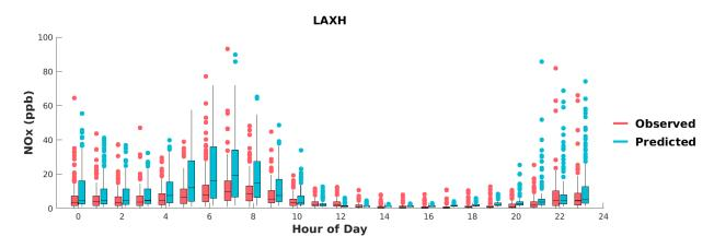
FIGURE I-11: BOX PLOTS OF OBSERVED VS. PREDICTED HOURLY NOX DURING MAY 1<sup>ST</sup> TO SEPTEMBER 30<sup>TH</sup>, 2018, AT LAX. HORIZANTAL LINES INDICATE 25<sup>TH</sup>, 50<sup>TH</sup> (MEDIAN), AND 75<sup>TH</sup> PERCENTILES.
