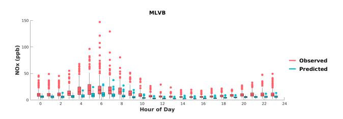
FIGURE I-12: BOX PLOTS OF OBSERVED VS. PREDICTED HOURLY NOX DURING MAY 1<sup>ST</sup> TO SEPTEMBER 30<sup>TH</sup>, 2018, AT MIRA LOMA VAN BUREN. HORIZANTAL LINES INDICATE 25<sup>TH</sup>, 50<sup>TH</sup> (MEDIAN), AND 75<sup>TH</sup> PERCENTILES.
