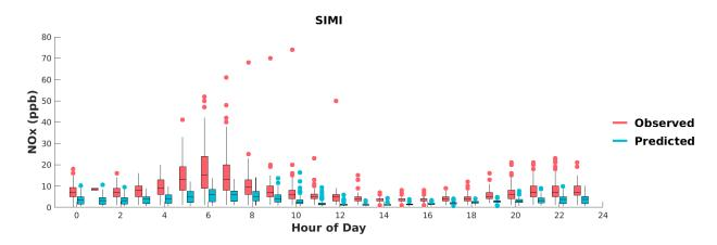
FIGURE I-20: BOX PLOTS OF OBSERVED VS. PREDICTED HOURLY NOX DURING MAY 1<sup>ST</sup> TO SEPTEMBER 30<sup>TH</sup>, 2018, AT SIMI VALLEY. HORIZANTAL LINES INDICATE 25<sup>TH</sup>, 50<sup>TH</sup> (MEDIAN), AND 75<sup>TH</sup> PERCENTILES.
