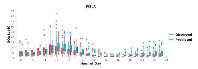
FIGURE I-23: BOX PLOTS OF OBSERVED VS. PREDICTED HOURLY NOX DURING MAY 1<sup>ST</sup> TO SEPTEMBER 30<sup>TH</sup>, 2018, AT WEST LOS ANGELES. HORIZANTAL LINES INDICATE 25<sup>TH</sup>, 50<sup>TH</sup> (MEDIAN), AND 75<sup>TH</sup> PERCENTILES.
