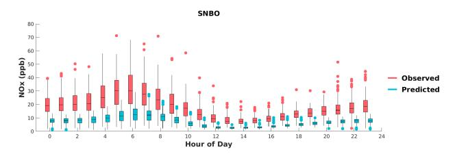
FIGURE I-21: BOX PLOTS OF OBSERVED VS. PREDICTED HOURLY NOX DURING MAY 1<sup>ST</sup> TO SEPTEMBER 30<sup>TH</sup>, 2018, AT SAN BERNARDINO. HORIZANTAL LINES INDICATE 25<sup>TH</sup>, 50<sup>TH</sup> (MEDIAN), AND 75<sup>TH</sup> PERCENTILES.
