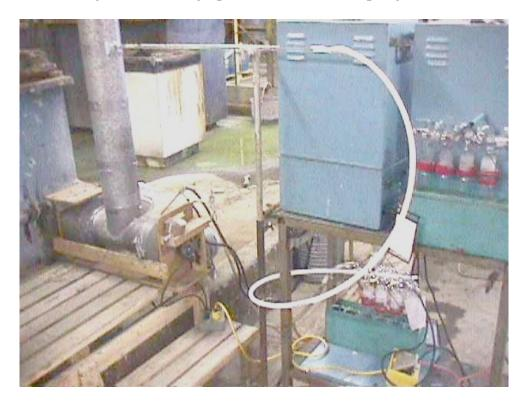
Figure 4 – Photograph of Chromium Sampling System.
