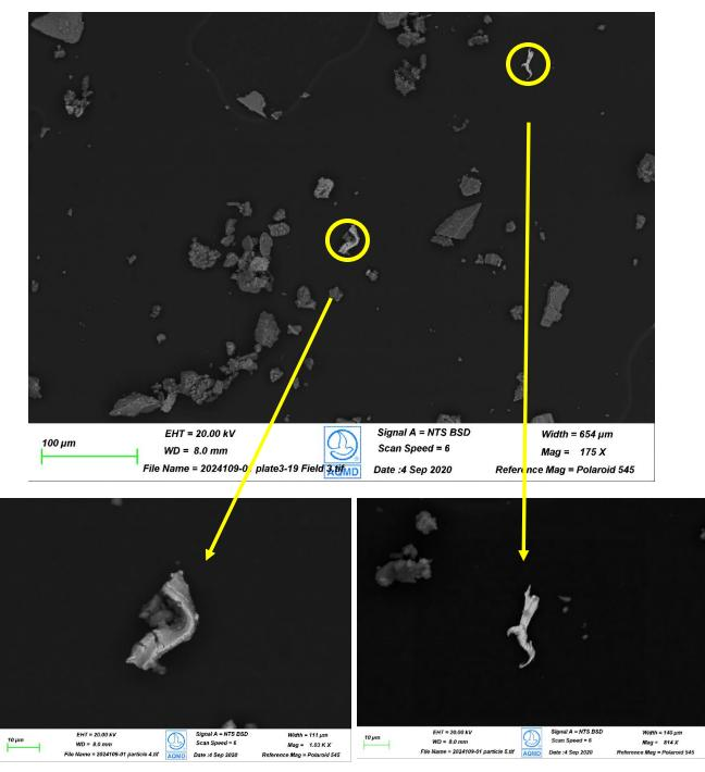
**Figure 2.** Southeast Middle School: Two metallic particles containing Cr and other metals. Composition, shape and surface texture resemble particle from metal grinding or shaving.
