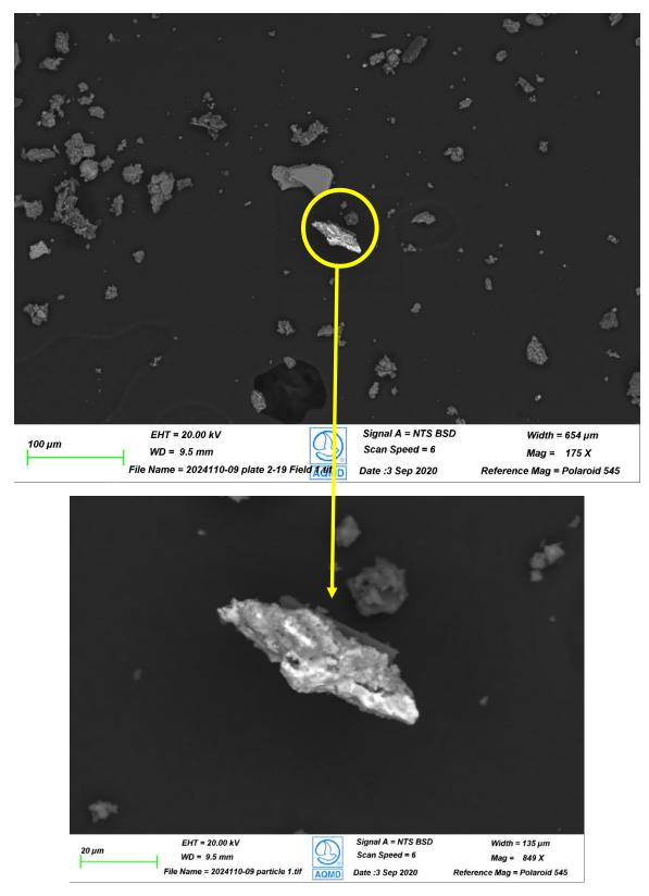
Figure 4. Westside #2: Amorphous Pb containing particle.
