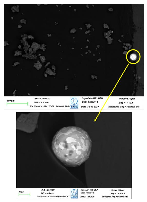
**Figure 3.** Westside #1: Spherical particle containing Pb and Sn. Composition, shape and surface texture resemble particle formed from a hot process such as soldering/welding.
