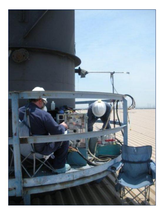
Figure 6: CARB Method 436 Field Sampling Train and Probe
