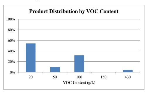
**Figure 6 – Adhesive - Subfloor Adhesives**
