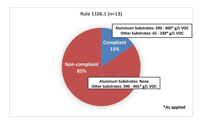
FIGURE 1-2: TOPSIDE COATINGS SUBJECT TO EXISTING RULE 1106 AND 1106.1 VOC LIMITS USED AT SHIPYARDS, BOATYARDS AND MARINAS VISITED BY SCAQMD STAFF
