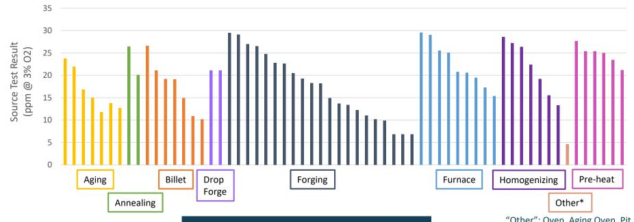
All furnace types have a source test result < 25 ppm
