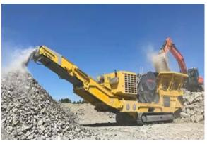
concrete/asphalt/stone demolition materials into smaller sized recycled aggregate for re-use. Figure 1-3 shows a similar inactive portable crusher located at a roadway project near a receptor fence line.
