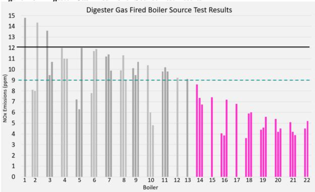
Figure 2-3 – Digester Gas Fired Boiler Source Test Results
