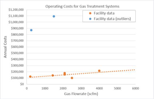
Figure 4-2 – Operating Costs for Gas Treatment Systems
