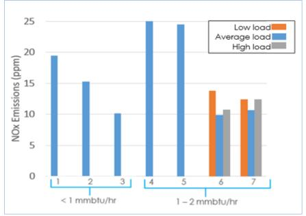
Figure 2-2 – Digester Gas Boiler Source Test Results
