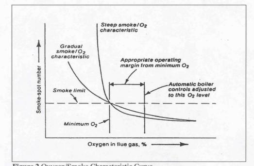
Figure 2 Oxygen/Smoke Characteristic Curve
