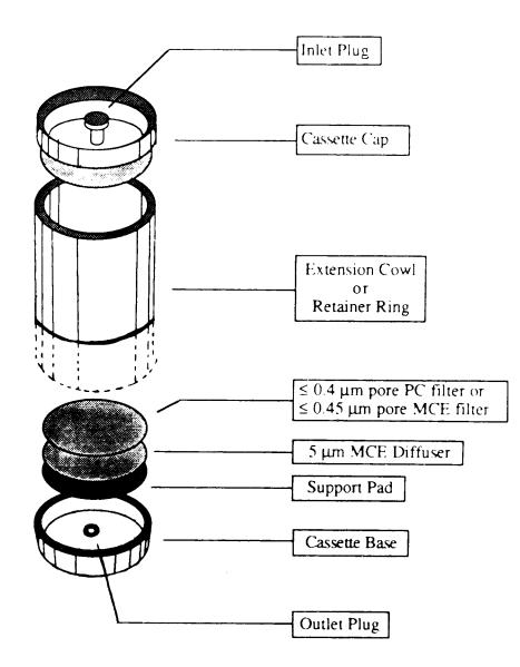
h. When polycarbonate filters are used, position the highly reflective face such that the incoming particulate is received on this surface. i. Seal the cassettes to prevent leakage around the filter edges or between cassette part joints. A mechanical press may be useful to achieve a reproducible leak-free seal.
