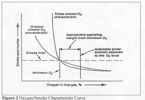
7. From the curves prepared in Step 6, find the stack gas oxygen levels where the CO emissions or smoke-spot number equal the following values:
