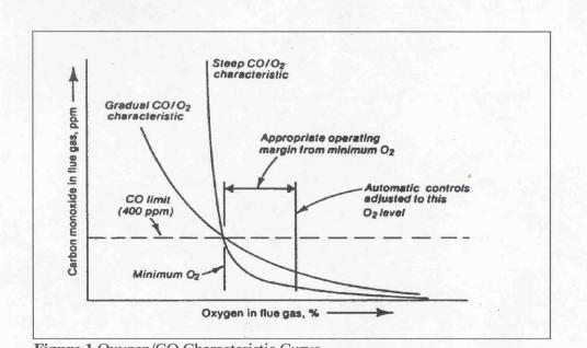
Figure 1 Oxygen/CO Characteristic Curve
