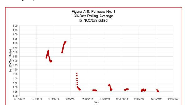
Figures A-9 illustrates the NOx emissions on a rolling 30-day average based on the ratio of emissions to glass pulled for the sodium silicate furnace from CY 2016 to CY 2019.
