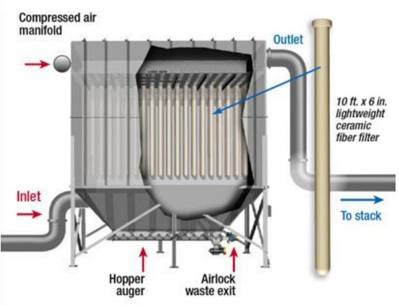
Figure 2-3: Tri-mer Ultracat Control System Baghouse\*
