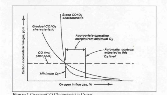
Figure 1 Oxygen/CO Characteristic Curve
