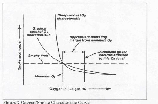
Figure 2 Oxygen/Smoke Characteristic Curve
