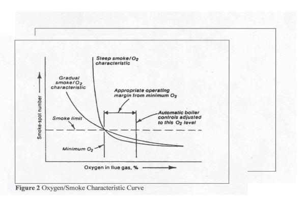
7. From the curves prepared in Step 6, find the stack gas oxygen levels where the CO emissions or smoke-spot number equal the following values:
