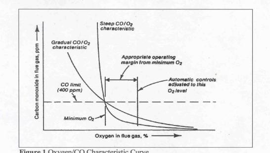
Figure 1 Oxygen/CO Characteristic Curve
