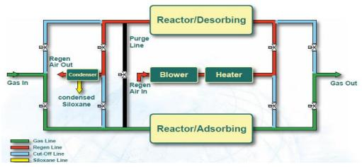
Figure 2. DCL Biogas Treatment System
