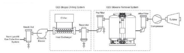
Figure 8. Typical Parker GES Landfill Gas Flow Schematic
