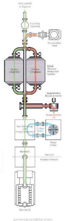
Figure 1. Willexa Biogas Treatment System
