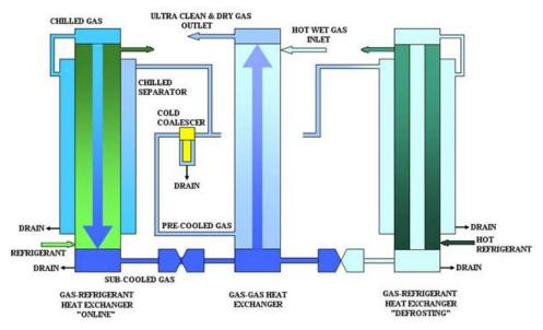
Figure 3. Pioneer Total Contaminant Removal (TCR) System
