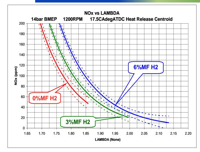
Lambda at the limit of combustion stability was observed to be as follows:
