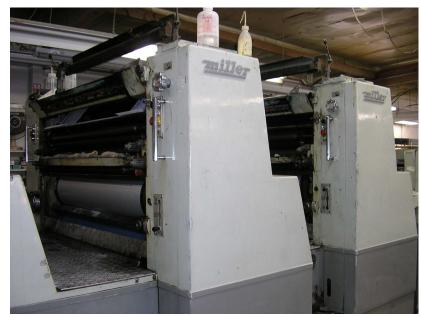
Figure 2-15. Two Color Press at The Printery
