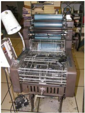
Figure 1-2. Rollers on Small Lithographic Press
