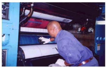
Figure 1-1. Blanket on lithographic printing press
